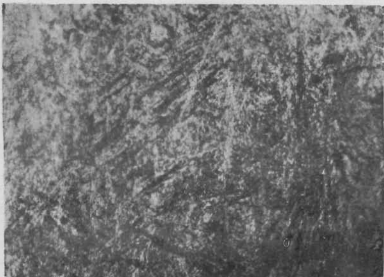
Photomicrograph VI (X145) MICROSTRUCTURE AT THE CUTTING EDGE OF AN AXE
